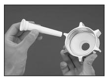
Figure 5. Sausage stuffing cone installation
